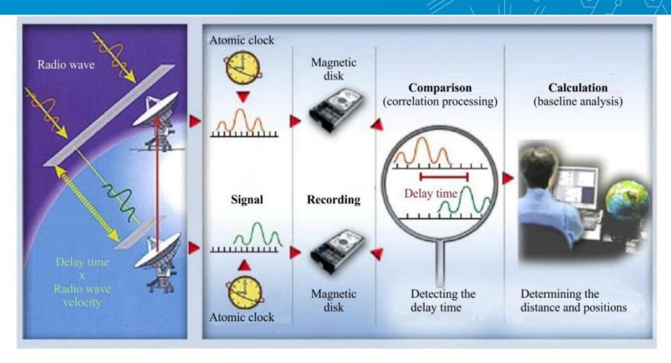
VLBI is a fundamental geodetic technique that underpins high accuracy positioning by observing weak cosmic radiation using a global network of radio telescopes.
