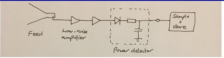
Simple radiometer – not useful in practice because amplifiers are not stable
