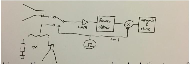
Switching radiometer – measures signal relative to a reference, through the same amplifier
