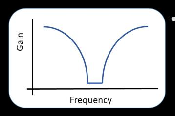
Persistent RFI typically only affects a narrow frequency band. Therefore a common method to improve the S/N is to use narrow band rejection filters (or 'notch filters') to block radio frequency bands known to contain high levels of interference.
